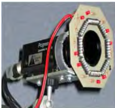
Fig. 1. A camera with a system emitting infrared light and an infrared filter (source: own)
